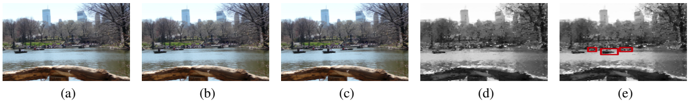
Fig. 6. (a) Original image (b) watermarked image (c) tampered image (d) reconstructed image using extracted watermark and (e) tampered region detection.
